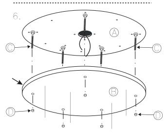
Remove rods and attach (a) to (b) with the button head screws (b)
